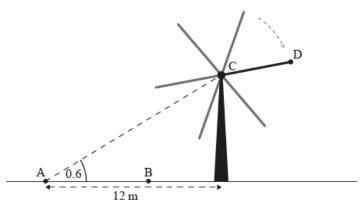
From point A the angle of elevation of point C is 0.6 radians.
