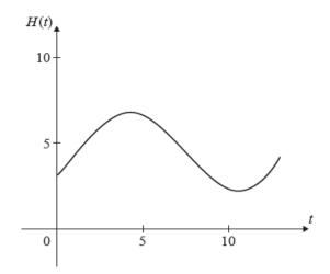
The first high tide occurs at 04:30 and the next high tide occurs 12 hours later. Throughout the day, the height of the water fluctuates between 2.2 m and 6.8 m.
