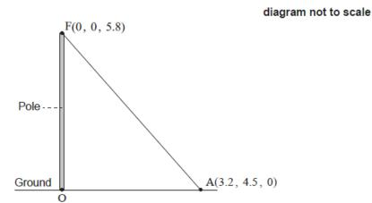
The pole is held in place by ropes attached at F.
